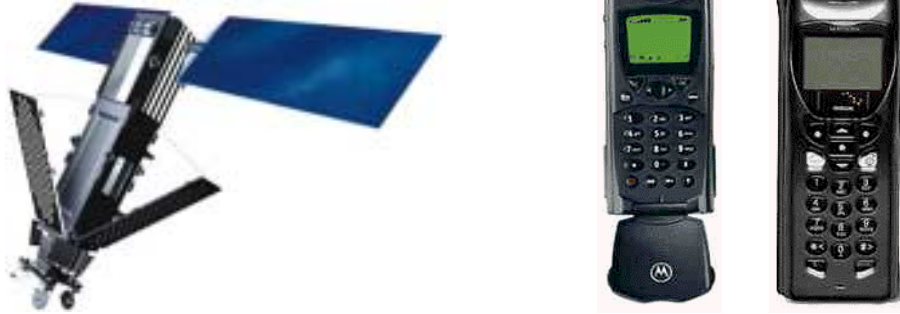
Figure 10. (left) Individual Iridium satellite in deployed on-orbit configuration (right) Motorola and Kyocera Iridium handheld satellite telephones
