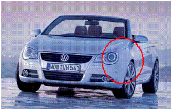
Figure 1. Volkswagen Eos and Eos fender. An example of a stamped steel part.
