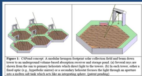
Figure 1: CSPond concept. A modular hexagonal footprint solar collection field and beam down tower to an underground volume-based absorption receiver and storage pond. (a) Several rays are shown from the sun to primary heliostats which direct light to the towers. (b) In each tower, either a fixed optic (e.g., hyperbolic mirror) or a secondary heliostat focuses the light through an aperture into a molten salt tank which acts like an integrating sphere. (patent pending)
