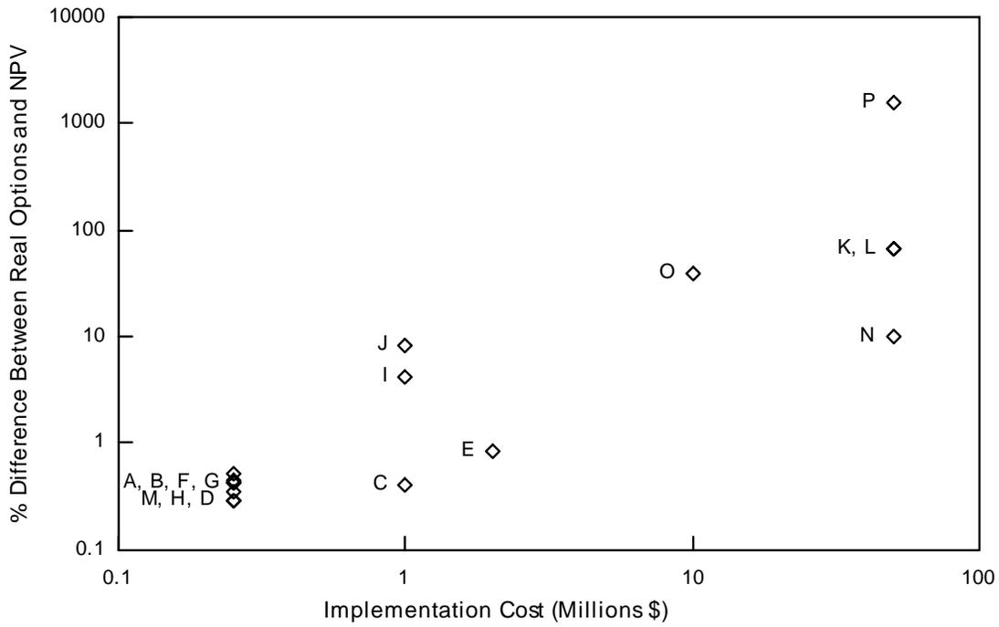
**Figure 5: Flexibility in Product development, specifically the option to drop a project, increases in value as the relative cost of the implementation in Stage 2 becomes larger compared to Stage 1.**
