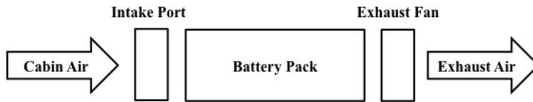
**Figure 6.1: Sealed-cabin-air cooling**
