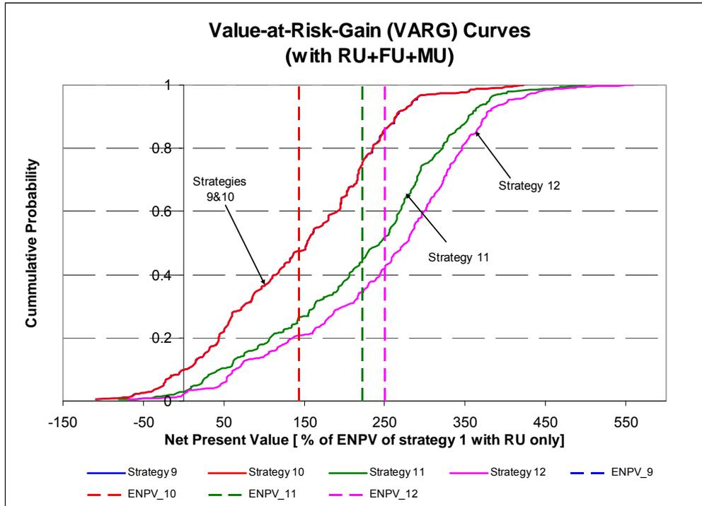
Figure 6.5: Dominant target curves. Strategies 11 and 12 for design of oil platform complex dominate Strategy 1. (Horizontal normalized to preserve commercial confidentiality) (Source: Lin, 2009)
