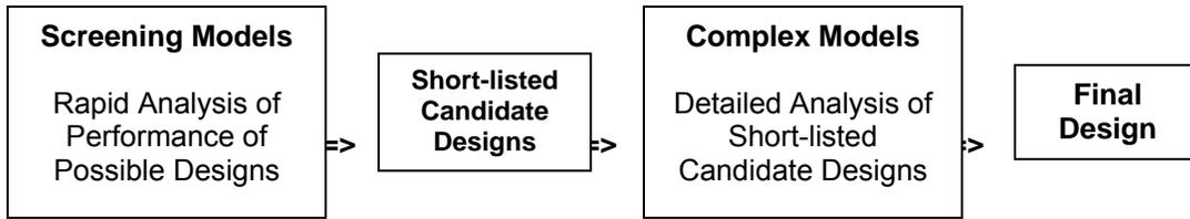
Figure 5.1: Screening Models Precede and Complement Detailed Design Models
