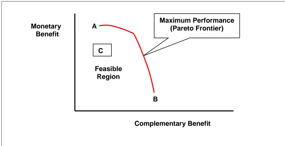
Figure 6.7: General diagram of the performance of designs when all axes represent benefits. In this case, the set of best designs, known as the Pareto frontier, is furthest away from the origin.
